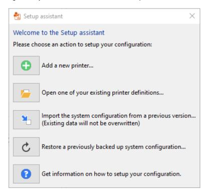
The "Import the system configuration from a previous version" option allows you to transfer your former user-defined settings (including printer definitions, program settings, job data, profiles and linearizations) directly to the new version e.g., after updating the software - without the need to manually backup and then restore the system configuration.
